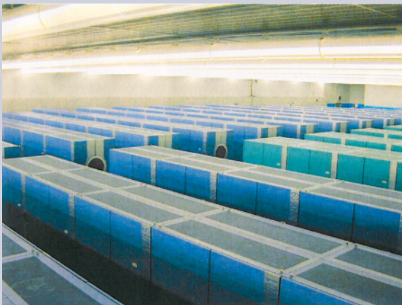
FIG. SB1. The Earth Simulator machine of the Frontier Research Project. The machine is located in Yokohama, Japan. Its measured performance is 35.61 Tflops. It consists of 640 nodes that are connected by a high-speed network. Each node contains eight vector processors with 16 GB of memory, for a total of 5120 processors and 10 TB of memory. The Earth Simulator is capable of running a super-GCM fast enough to enable practical climate change simulations.
