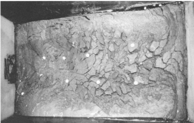
Figure 2: 1/20 scale centrifuge model of a shallow translational landslide developed during thaw of a 24° slope formed in frozen overconsolidated silty clay. Thawing took place under gravitational acceleration of 20g. Test box length is 750 mm, which scales to a prototype length of 15 m. The model thickness is 90 mm, scaling to 1.8 m and the slip surface depths are approximately 30 mm and 50 mm, equivalent to 0.6 m and 1.0 m at prototype scale. (a) Side view. Note two adjacent arcuate slip scars on right of photograph and corresponding lobate toe zones on the left of the photograph; (b) Plan view. The twin arcuate slip scars are clearly visible on the right of the photograph. White discs are plastic displacement markers in the central part of the model where displacements were least.
