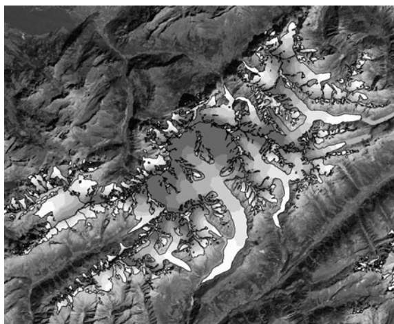
Fig. 6. Glacier extent for the Aletsch region in 1973 (black outlines) and modelled extent for six shifts of the steady-state ELA using an AAR of 0.6. The legend gives the greyscale that will disappear due to the corresponding shift in ELA. For an ELA rise of 600 m, only the darkest regions will remain. The background is a Landsat satellite image acquired at 31 August 1998. Landsat data © Eurimage/Swiss National Point of Contact for Satellite Images (NPOC).
