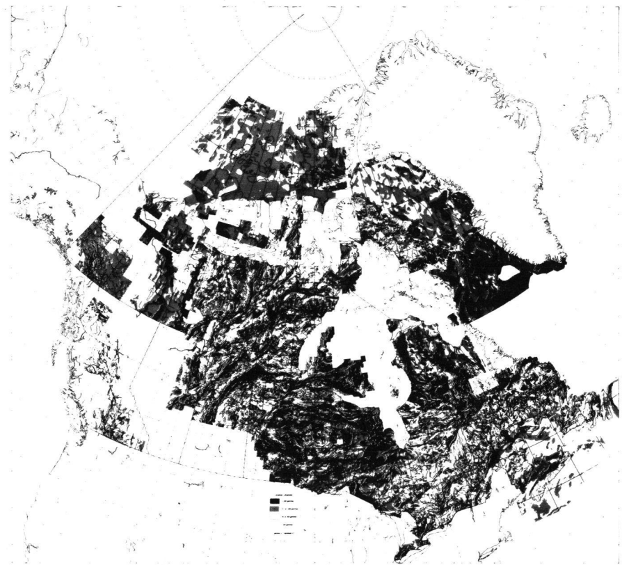
Fig. 3. Composite aeromagnetic map of Canada, compiled by the Geological Survey of Canada (1960-1985). Dark tones indicate positive anomalies, while light tones show negative anomalies.
