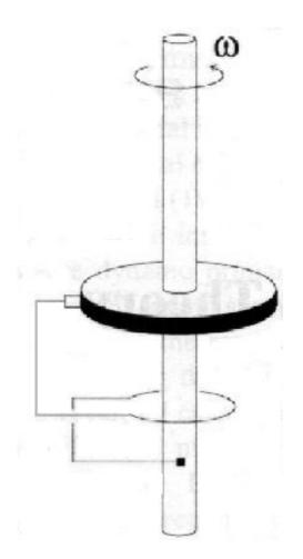
Figure 1: Single-disc dynamo, from Merrill
