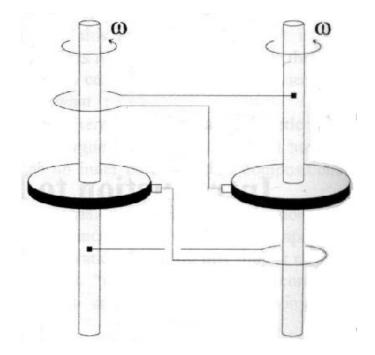
Figure 3: Two-disc dynamo, from Merrill
