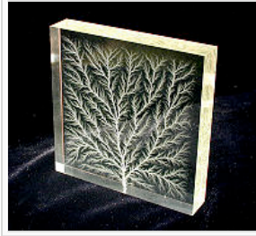
High voltage breakdown within a 4" block of acrylic creates a fractal Lichtenberg figure.
