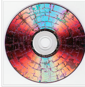
Fractal branching occurs in a fractured surface such as a microwave-irradiated DVD. [9]
